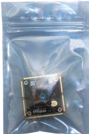
Place Camera Sample into Anti-Static Bag
